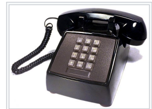
The Western Electric No. 2500, a typical American 12-button phone of the 1970s and early 80s
